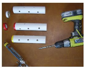
Figure 4. Holes drilled in PVC pipe.
