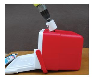
Figure 2. Drilling at an angle with hole saw.
