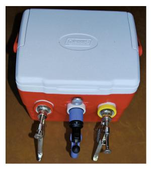
Figure 6. Finished syringe cooler. The best way to make sure a cooler is ready for use is to slide one or two thawed ice packs under the PVC pipe, place the unit in a freezer, let the ice packs freeze. When ready to use, place another ice pack on top of the PVC to ensure the syringes stay cold. If ice is used, make sure the water level from melting ice does not reach the bottom of the PVC pipe and contaminate the needle ends.
