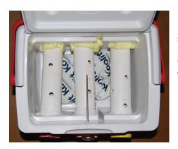
Figure 5. Inside of syringe cooler with probe thermometer in center.
